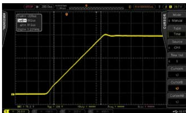
DC Voltage Ramp Up @ 100Vdc/ms programmed slew rate Captured
