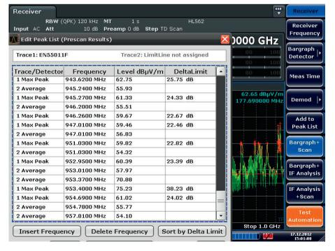
Results of standard-compliant final measurements presented in tabular format, stating the offset values (deltas) with respect to the applicable limit values. Results can be exported as an ASCII file for further processing.
