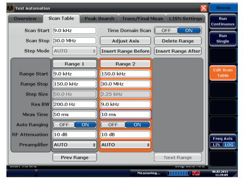
In receiver mode, the R&S°ESRP is tuned across a user-defined frequency range in line with the settings made in the scan table. Users can define up to ten frequency subranges and configure the parameters independently for each subrange (for example range start/stop, step size, measurement time, resolution bandwidth, input attenuation).
